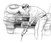
Step 9: PUT WIRE ROPE UNDER TENSION. Using the winch switch, slowly wind the wire rope until no slack remains. Once the wire rope is under tension, stand well clear, and never step over it.
