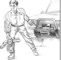
Step 4: PULL WIRE TO ANCHOR POINT. Pull out enough wire rope to reach your anchor point. Be sure to keep a certain amount of tension in the wire. It can become twisted and overwrap when slackened, leading to wire rope damage. To prevent loosing the end, hold the winch hook in the hook strap
