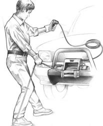
**Step 18:** REWIND WIRE ROPE. The person handling the wire rope should walk the rope in and not let it slide through the hand and control the winch at all times.
